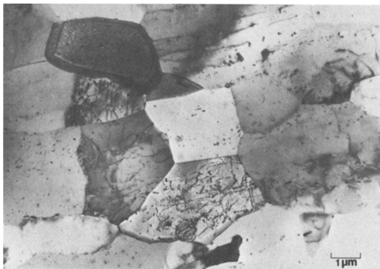
Figure 5 The microstructure observed after 100% superplastic deformation at 490^\circ\text{C} , \dot{\epsilon} = 10^{-3} \text{ sec}^{-1} (Region II). It can be seen that the structure is relatively equiaxed, but with a highly variable dislocation density.
